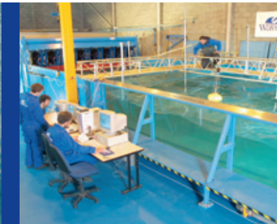
Wave tank to simulate wave conditions
