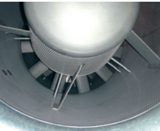
100 kW Wells turbine
